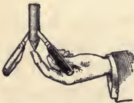
FIG. 34.—A System in Stable Equilibrium.
